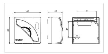
Electrical contact capacity = 16(2,5) A / 250 Vac Regulation range = 5°÷30°C
