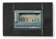
FAN 503 is an electronic built-in DIN503 regulator for fan coils, radiators and fan convectors with LCD display. It includes three relays to regulate the fan speed and two relays to control the solenoid valves and the water probe inlet (NTC 10K probe included in the package).
