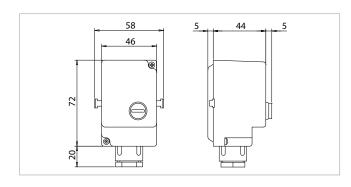
Temperature limiter pre-regulation =  $60^{\circ}$ C Regulation range =  $40^{\circ}$ ÷ $70^{\circ}$ C Tolerance = 0-10K Manual reset Reset temperature = -25K ± 8K range Max. head temperature =  $55^{\circ}$ C Electrical contact capacity = C-1: 0,5 A / 250 Vac C-2: 10(2,5) A / 250 Vac Protection rating = 1P40 Certifications = CE, ENECO3, EAC
