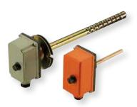
LSC1 is a boxed immersion thermostat, with liquid expansion probe, unipolar, safety temperature limiter with manual reset, fail-safe for capillary breakage, complete with watertight protection pocket. Useful in appliances where safety is required due to the temperature increase.
