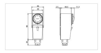
Differential = 8±3K Electrical contact capacity = 16(2,5) A / 250 Vac Thermal gradient = 1°K/min. Max. head temperature = 80°C Protection rating = IP20 Certifications = CE, ENECO3, EAC
