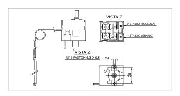
Electrical contact capacity = 15 (2,5) A / 250 Vac Switches = changeover Max. head temperature = 80°C Capillary length = 1500 mm PVC Min. capillary curvature radius = 5 mm Connection = via faston Certifications = CE, ENECO3, EAC
