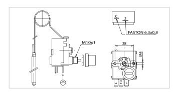
Switches = interrupted due to temperature increase Max. head temperature = 85°C
