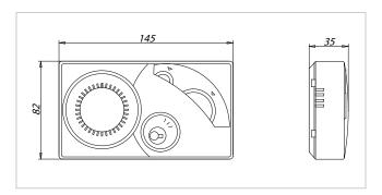
Electrical contact capacity = 5(1) A / 250 Vac Temperature range = 10°÷30°C Differential = 0.5 K Insulation class = II Protection rating = IP20 Max. room temperature = 50°C Power supply =  $2 \times 1.5V-LR6$  AA batteries Operating mode: Manual / Automatic Heating system
