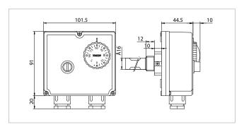
Electrical contact capacity = 10 (2,5) A / 250 Vac Switches = interrupted due to temperature increase or exchange Max. head temperature = 80°C Max. bulb temperature = 125°C Thermal gradient = 1°K/min Protection rating = IP40 Certifications = CE, ENECO3, DIN, PED, EAC
