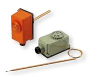
TC2 is a boxed immersion thermostat with liquid expansion, unipolar, with changeover switches, complete with a watertight protection pocket. The thermostat normally applied on delivery piping is particularly suitable for the automatic regulation of boilers, pumps and other various appliances. It is also available in a capillary version.
