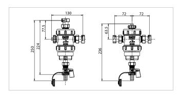
Max pressure = 3 bar Max. temperature =  $0 \div 90^{\circ}$ C Compatible fluids = Water and non-aggressive fluids Connections:  $G3/4^{\circ}$  ISO228/1 female swivel captive nut hose fitting Ø15 mm Certifications = CE
