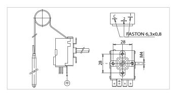
Electrical contact capacity = NC 16(6) / A 250 Vac Switches = changeover Max. head temperature = 85°C Min. capillary curvature radius = 5 mm Connection = via faston 6,3x0,8 Certifications = CE, ENECO3, EAC, UL, CSA
