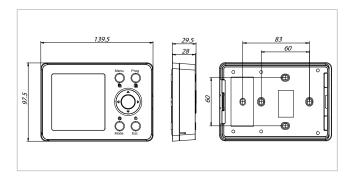
Electrical contact capacity = 5(1) A / 250Vac Regulation range = 5°÷35°C  $N^{\circ}$  of settable temperatures = 3 Time slots = 0.5 hDifferential = 0,2 K Thermometer resolution =  $0,1^{\circ}C$ Thermometer precision =  $\pm 0.3$ °C Max. room temperature = 50°C Insulation class = II Protection rating = IP20 Options = 12h/24h clock and °C/°F selection Operating mode: Manual/Automatic/Anti-freeze System: heating/air conditioning Certifications = CE, ENECO3, EAC
