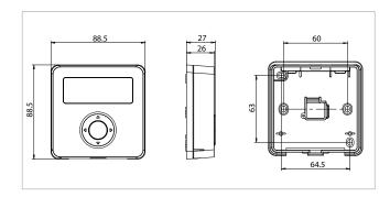
Electrical contact capacity = 5(1)A / 250 Vac Regulation range = 5°÷35°C
