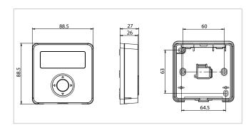
Electrical contact capacity = 5(1) A / 250 VacRegulation range = 5°÷35°C  $N^{\circ}$  of settable temperatures = 2 Time slots = 1 hDifferential = 0,2 K Thermometer resolution =  $0,1^{\circ}C$ Thermometer precision =  $\pm 0.3$ °C Max. room temperature = 50°C Insulation class = II Protection rating = IP20 Options = 12h/24h clock and °C/°F selection Operating mode: Manual/Automatic/Anti-freeze System: heating/air conditioning Certifications = CE, ENECO3, EAC
