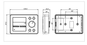
Electrical contact capacity = 5(1) A / 250 Vac Regulation range = 5°÷35°C  $N^{\circ}$  of settable temperatures = 2 Time slots = 0.5 h e 1 hDifferential = 0,2 K Thermometer resolution =  $0,1^{\circ}C$ Thermometer precision =  $\pm 0.3$ °C Max. room temperature = 50°C Insulation class = II Protection rating = IP20 Options = 12h/24h clock and °C/°F selection Operating mode: Manual/Automatic/Anti-freeze System: heating/air conditioning Form of control: TPI (optional) Certifications = CE, ENECO3
